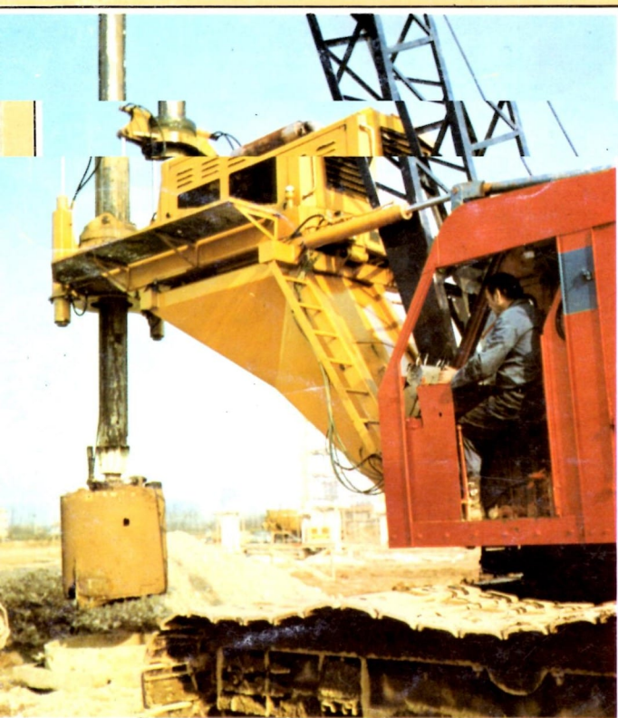
RT3-S con utensile bucket e trivella. / RT3-S with auger and bucket tools.
